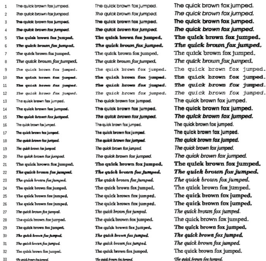
Fig. 4.7 Bitmap rendering in 12, 14, and 18 point of 33 standard Postscript text fonts
